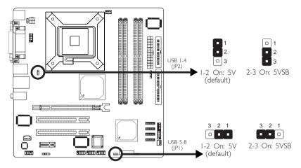
JPI and JP2 are used to select the power of the USB ports. Selecting 5VSB will allow you to use the USB keyboard or USB mouse to wake up the system.
