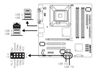
The system board supports 8 USB 2.0/1.1 ports. USB allows data exchange between your computer and a wide range of simultaneously accessible external Plug and Play peripherals.
