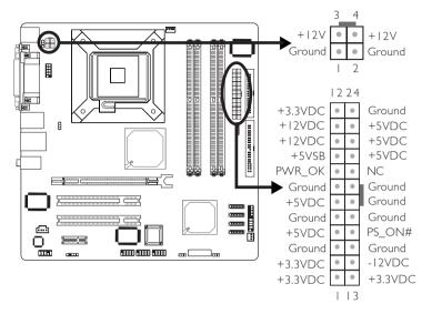
We recommend that you use a power supply that complies with the ATX12V Power Supply Design Guide Version I.I. An ATX12V power supply has a standard 24-pin ATX main power connector and a 4-pin +12V power connector that must be inserted onto CN8 and CN9 connectors respectively.
