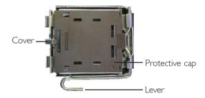
5. Lift the protective cap from the location pointed below to detach the cap from the cover.
