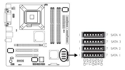
The system board is equipped with four Serial ATA connectors for connecting Serial ATA devices. Connect one end of the Serial ATA cable to J15 (SATA 1), J16 (SATA 2), J17 (SATA 3) or J18 (SATA 4) and the other end to your Serial ATA device.
