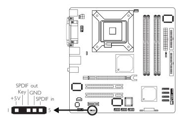
The system board is equipped with a S/PDIF connector. One cardedge bracket, mounted with S/PDIF ports, may be provided with the system board. Install the card-edge bracket to the system chassis then connect the audio cable connector to J5. Make sure pin 1 of the audio cable connector is aligned with pin 1 of J5.
