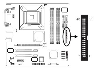
The system board is equipped with a shrouded PCI IDE header that will interface two Enhanced IDE (Integrated Drive Electronics) disk drives. To prevent improper IDE cable installation, the shrouded PCI IDE header has a keying mechanism. The 40-pin connector on the IDE cable can be placed into the header only if pin I of the connector is aligned with pin I of the header.
