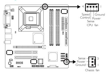
Connect the CPU fan's cable connector to the CPU fan connector (J8) on the system board. The chassis fan connector (J10) is used to connect an additional cooling fan. The cooling fan will provide adequate airflow throughout the chassis to prevent overheating the CPU and system board components.
