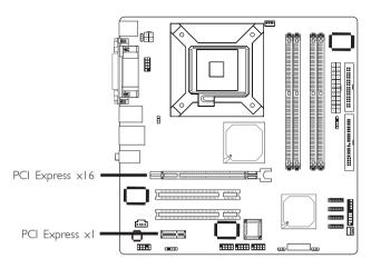
The system board is equipped with one PCI Express x16 and one PCI Express x1 slots.
