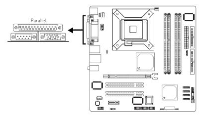
The system board has a standard parallel port (Burgundy) at location CN4 for interfacing your PC to a parallel printer. It supports SPP, ECP and EPP.
