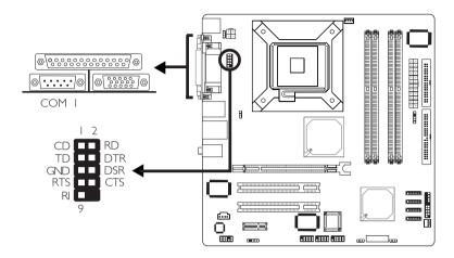
The system board is equipped with an onboard serial port (Teal/Turquoise) at location CN5 for COM I. It is also equipped with a 9-pin connector at location J9 for COM 2. The serial ports are RS-232C asynchronous communication port with I6C550A-compatible UARTs that can be used with a modem, serial printer, remote display terminal or other serial devices.
