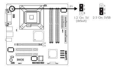
JP3 is used to select the power of the PS/2 keyboard/mouse port. Selecting 5VSB will allow you to use the PS/2 keyboard or PS/2 mouse to wake up the system.
