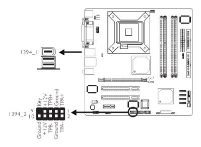
The system board is equipped with an onboard IEEE 1394 port at location CN1 (IEEE 1394\_I).
