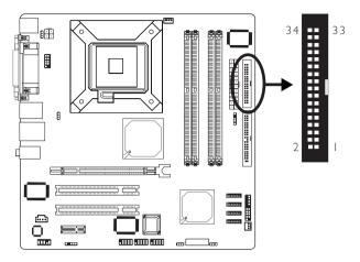
The system board is equipped with a shrouded floppy disk drive connector that supports two standard floppy disk drives. To prevent improper floppy cable installation, the shrouded floppy disk header has a keying mechanism. The 34-pin connector on the floppy cable can be placed into the header only if pin I of the connector is aligned with pin I of the header.
