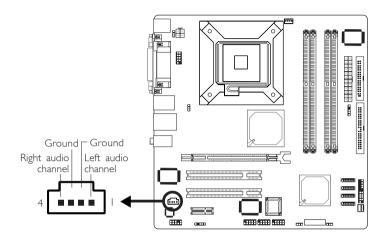
The CD-in (J6) connector is used to receive audio from a CD-ROM drive, TV tuner or MPEG card.
