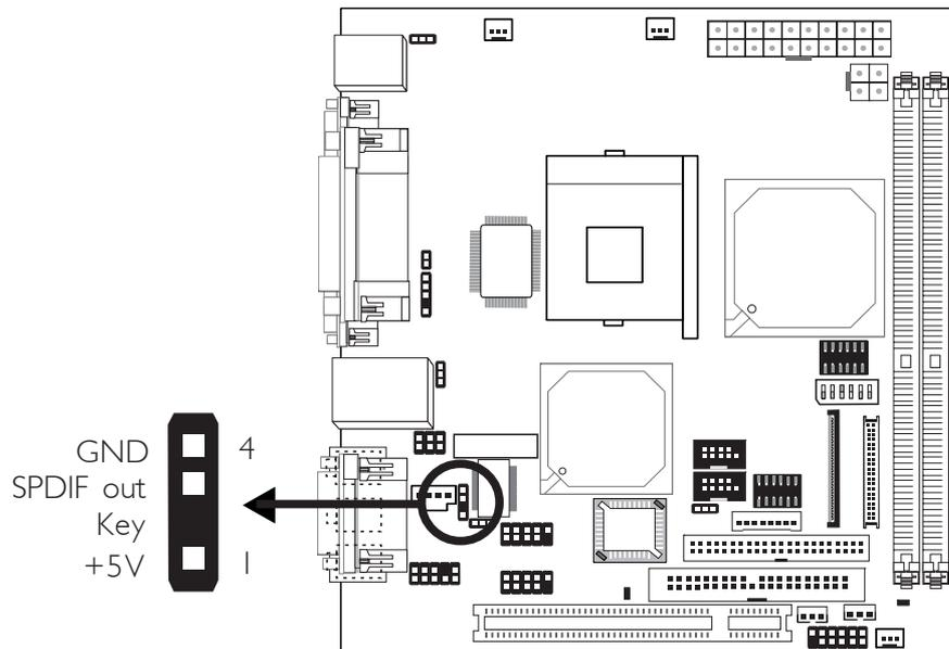
The S/PDIF-out connector (J7) is used to connect an external S/PDIF-out port. Your S/PDIF-out port may be mounted on a card-edge bracket. Install the card-edge bracket to the system chassis then connect the audio cable connector to J7. Make sure pin 1 of the audio cable connector is aligned with pin 1 of J7.
