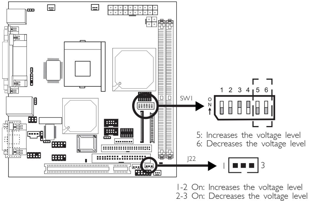
Use SW1's pins 5 and 6 or J22 to connect to the LCD Brightness Control button of the LCD Display Panel. It is used to adjust the brightness of the LCD Display Panel. Increasing or decreasing the voltage to control the LCD panel's brightness varies among Inverters. You must refer to the Inverter's specification to make the appropriate adjustment to the brightness of the LCD panel.
