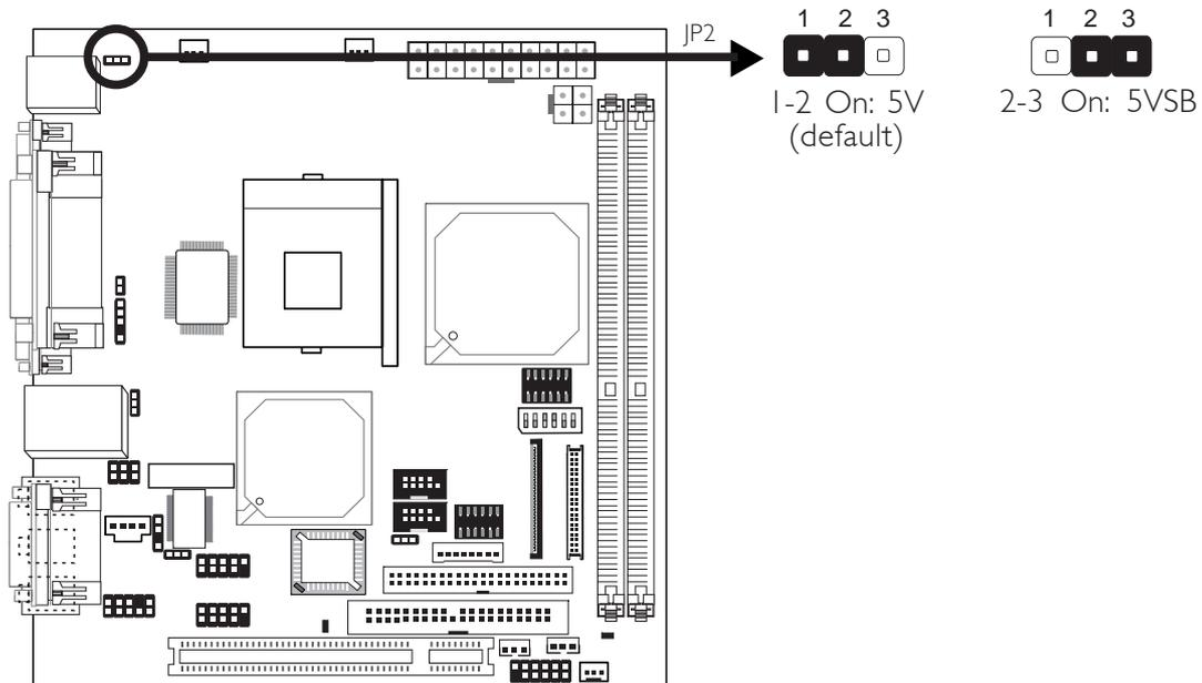
JP2 is used to select the power of the PS/2 keyboard/mouse port. Selecting 5VSB will allow you to use the PS/2 keyboard or PS/2 mouse to wake up the system.
