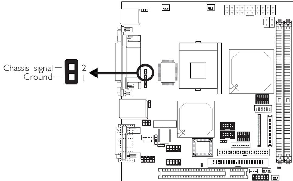
The system board supports the chassis intrusion detection function. Connect the chassis intrusion sensor cable from the chassis to J8. Whenever a chassis component has been removed, the sensor sends signal to J8 alerting you of a chassis intrusion event. To disable this function, place a jumper cap over J8.
