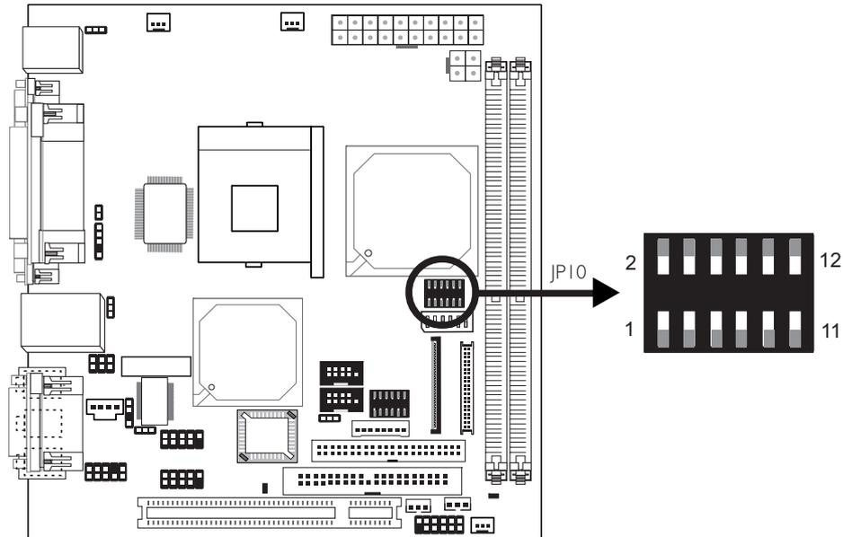
JPI0 is used to select the power supplied to the LCD panel as well as configure the inverter.
