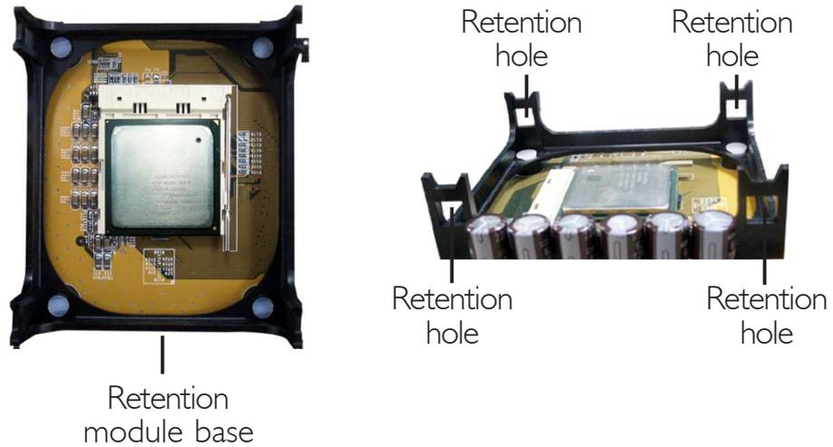
2. Position the fan / heat sink and retention mechanism assembly on the CPU, then align and snap the retention legs' hooks to the retention holes at the 4 corners of the retention module base.
