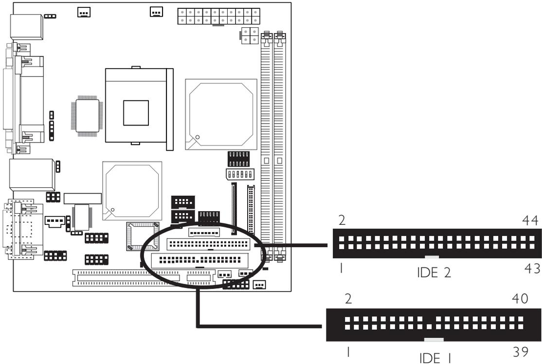
The system board is equipped with a 40-pin (IDE 1) and a 44-pin (IDE 2) IDE connectors. To prevent improper IDE cable installation, the IDE 1 connector has a keying mechanism. The connector on the IDE cable can be inserted into IDE 1 only if pin 1 of the cable connector is aligned with pin 1 of IDE 1.
