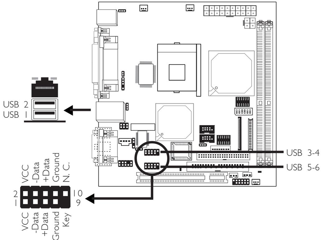
The system board supports 6 USB 2.0/1.1 ports. USB allows data exchange between your computer and a wide range of simultaneously accessible external Plug and Play peripherals.
