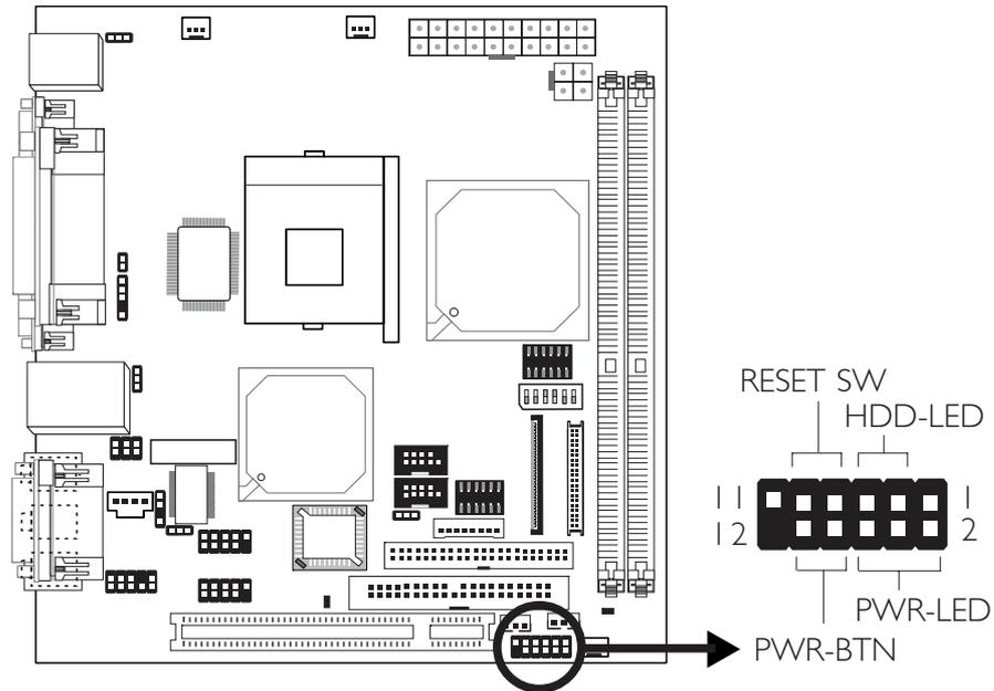
**HDD-LED - HDD LED**
