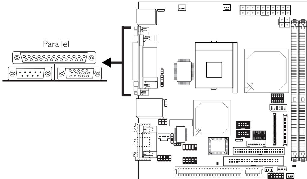
The system board has a standard parallel port (Burgundy) at location CN3 for interfacing your PC to a parallel printer. It supports SPP, ECP and EPP.
