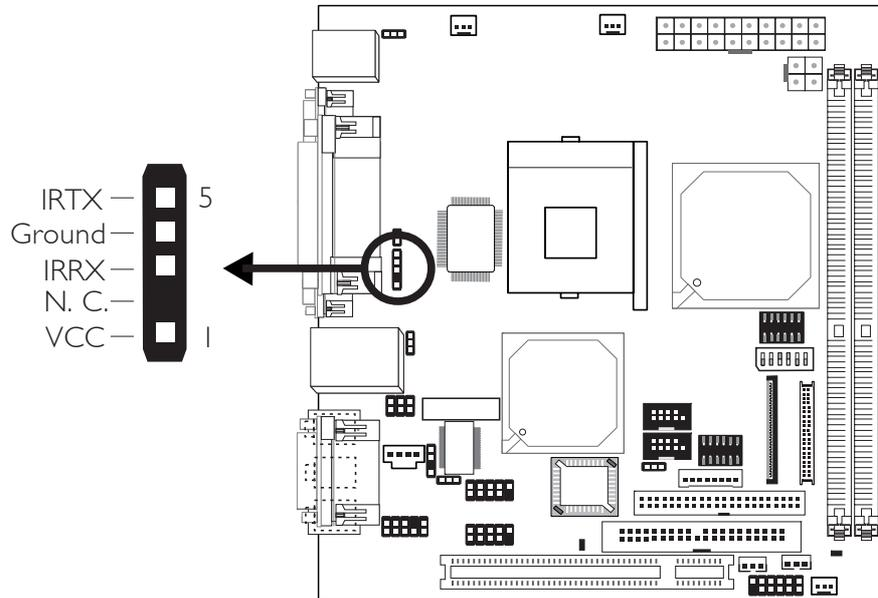
Connect your IrDA cable to connector J4 on the system board.
