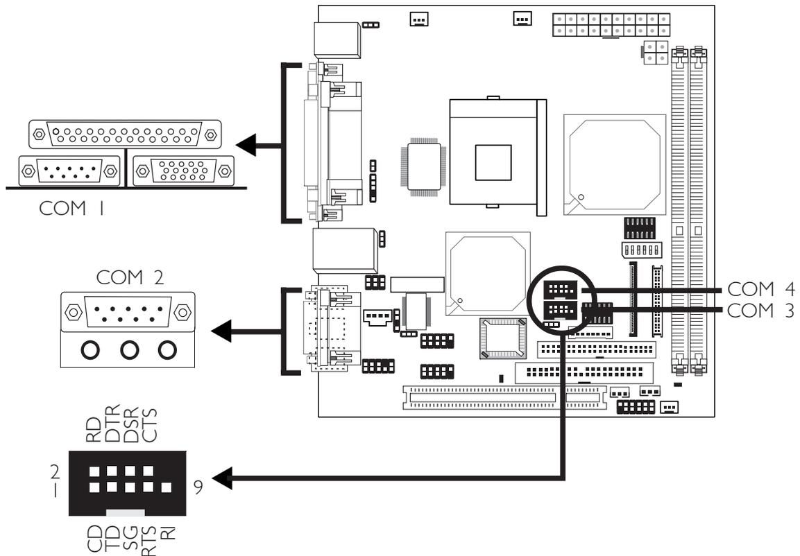
The system board is equipped with two onboard serial ports at locations CN13 (COM 1) and CN14 (COM 2). It is also equipped with two 9-pin connectors at locations J14 (COM 3) and J15 (COM 4). These serial ports are RS-232 and/or RS-485 asynchronous communication ports with 16C550A-compatible UARTs that can be used with modems, serial printers, remote display terminals, and other serial devices.
