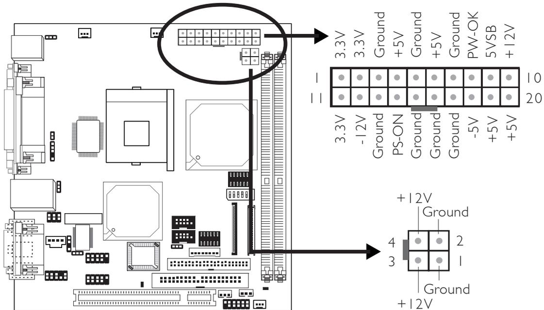
Use a power supply that complies with the ATX12V Power Supply Design Guide Version 1.1. An ATX12V power supply has a standard 20-pin ATX main power connector and a 4-pin +12V power connector that must be inserted onto CN10 and CN1 connectors respectively.
