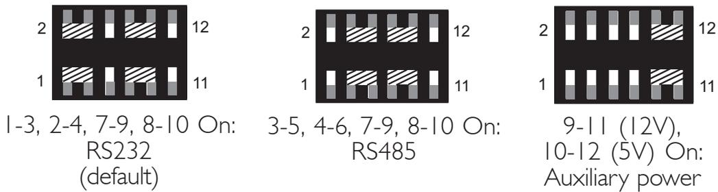
JP6 is used to set COM 4 to RS-232 or RS-485. If the serial device connected to this port requires 5V/12V power from the system board, set JP6 pins 9-11 and 10-12 to On. This setting automatically sets COM 4 at RS-232.
