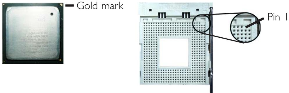
4. Insert the CPU into the socket until it is seated in place. The CPU will fit in only one orientation and can easily be inserted without exerting any force.
