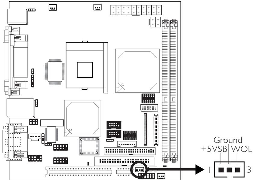
Your LAN card package should include a cable. Connect one end of the cable to the wakeup header on the card and the other end to location J12 on the system board. The network will detect Magic Packet and assert a wakeup signal to power-up the system. Refer to the add-in card's manual for details. Note: Your LAN card must support the remote wake up function.
