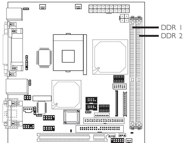
The system board supports DDR SDRAM DIMM. Double Data Rate SDRAM (DDR SDRAM) is a type of SDRAM that doubles the data rate through reading and writing at both the rising and falling edge of each clock. This effectively doubles the speed of operation therefore doubling the speed of data transfer.
