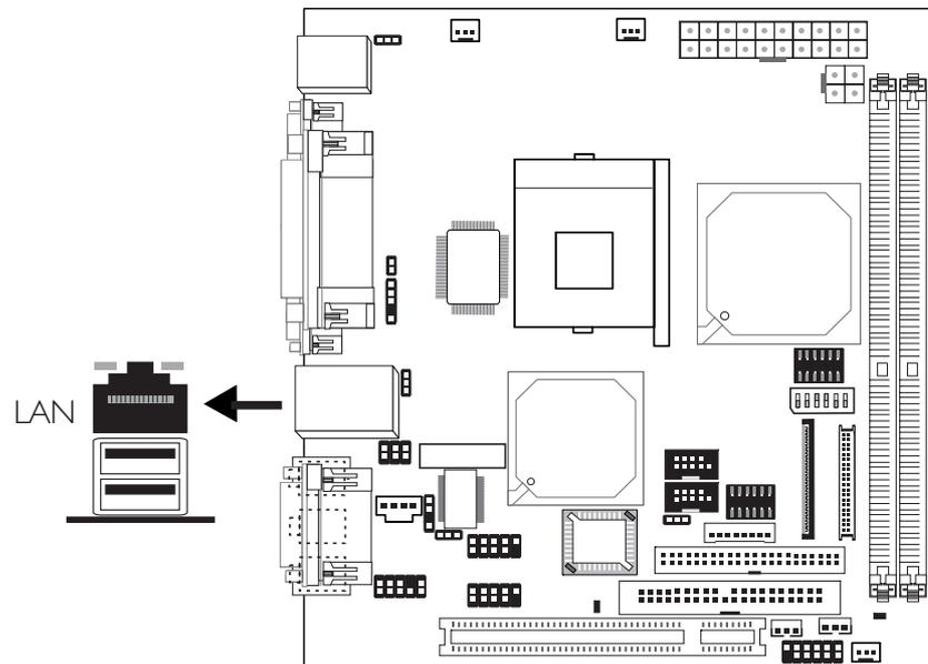
The system board is equipped with an onboard RJ45 LAN port. This port allows the system board to connect to a local area network by means of a network hub.
