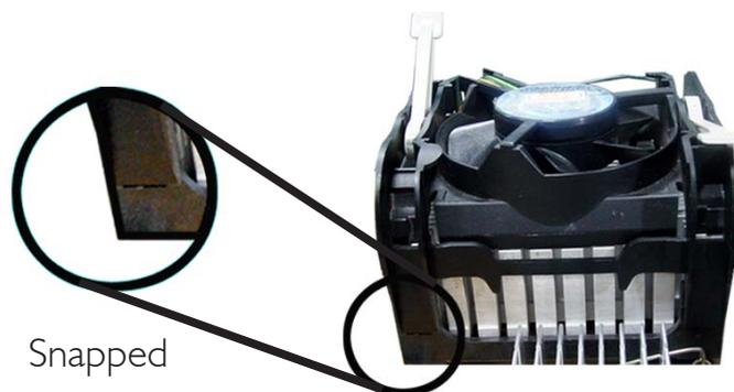
3. The retention levers at this time remains unlocked as shown in the illustration below.
