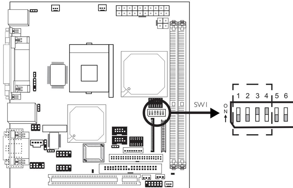
Set SWI pins 1 to 4 according to the type of LCD panel connected to the system. Please contact technical support for more information about the panel type settings.
