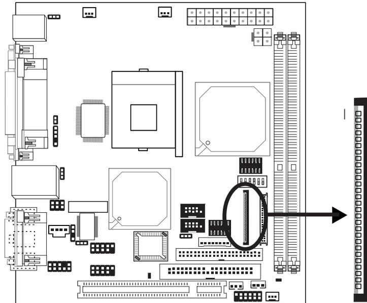
The system board is equipped with a 26-pin FPC type floppy disk drive connector. Only connect a 1.44MB slim-type floppy disk drive. Floppy drives other than the one mentioned above are optional. Refer to the next page for the pin function of this connector.
