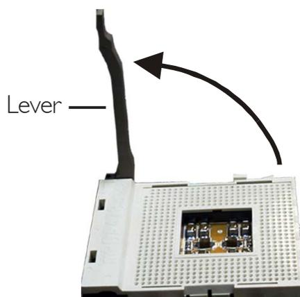
3. Position the CPU above the socket then align the gold mark on the corner of the CPU (designated as pin 1) with pin 1 of the socket.
