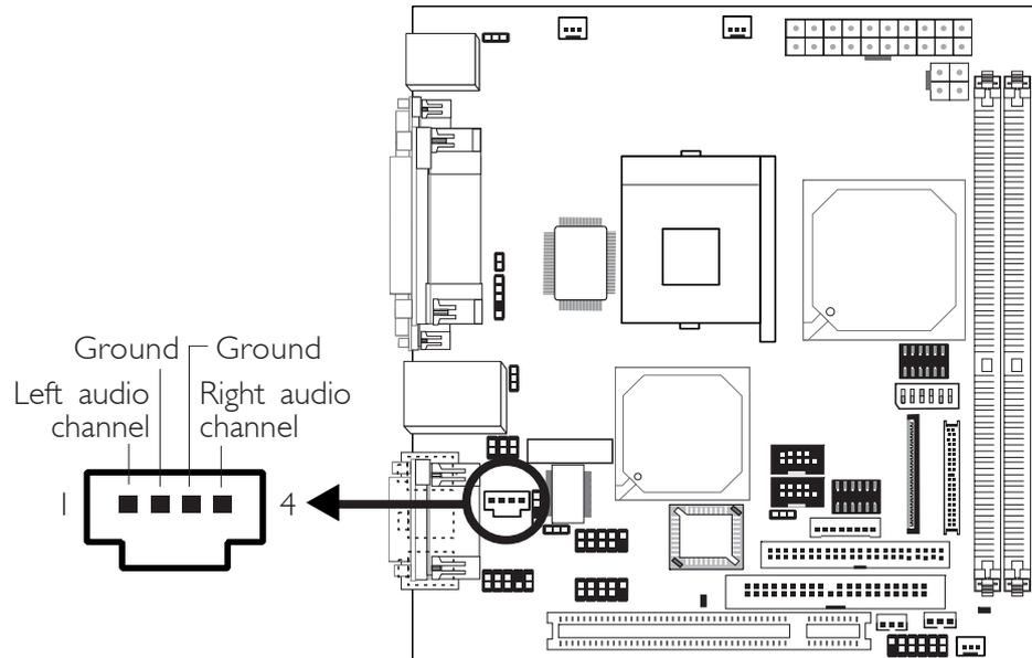
The CD-in (J5) connector is used to receive audio from a CD-ROM drive, TV tuner or MPEG card.
