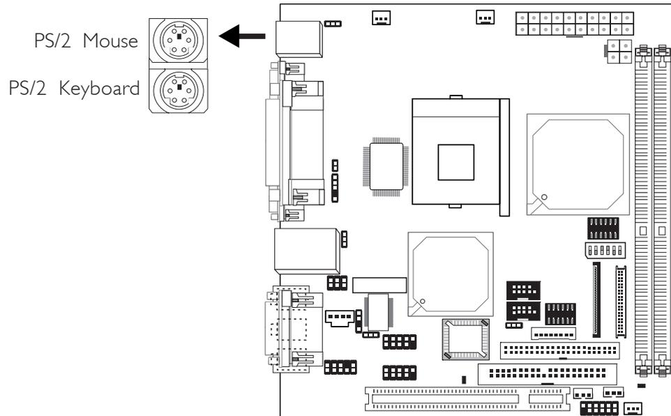
The system board is equipped with an onboard PS/2 mouse (Green) and PS/2 keyboard (Purple) ports - both at location CN5 of the system board. The PS/2 mouse port uses IRQ12. If a mouse is not connected to this port, the system will reserve IRQ12 for other expansion cards.
