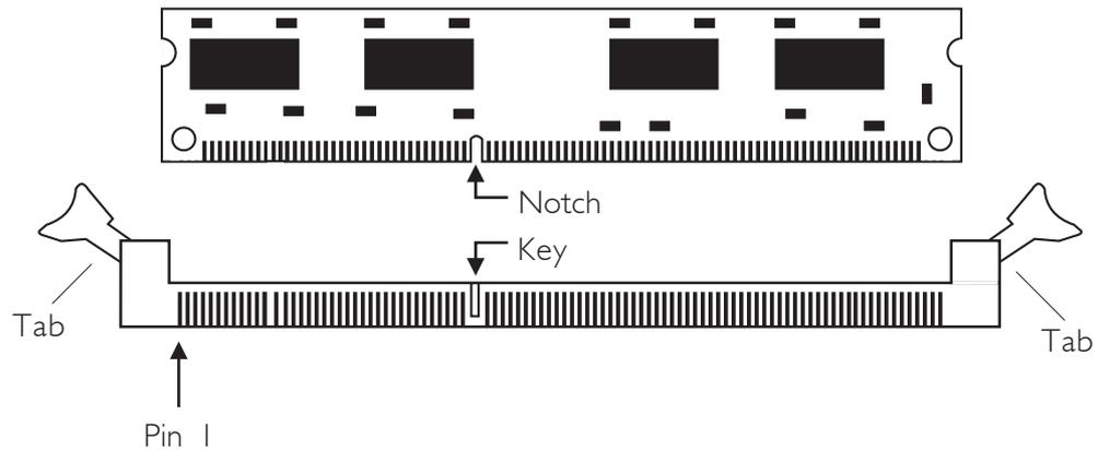
1. Pull the “tabs” which are at the ends of the socket to the side.
