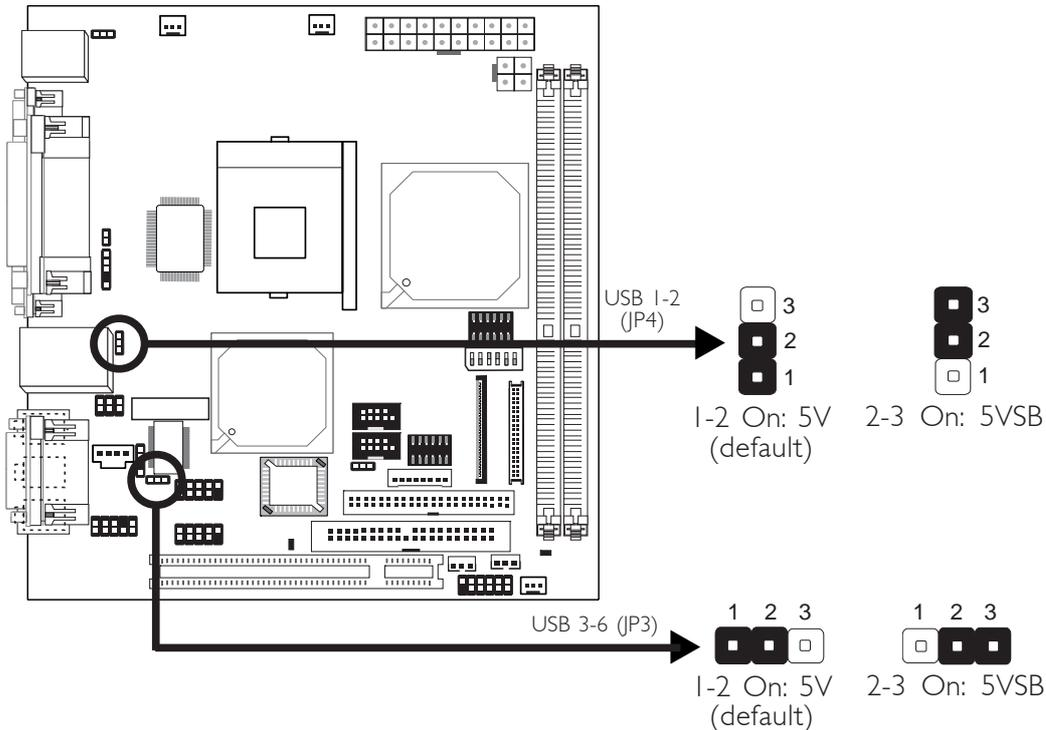
JP4 (for USB 1-2) and JP3 (for USB 3-6) are used to select the power of the USB ports. Selecting 5VSB will allow you to use the USB keyboard or USB mouse to wake up the system.
