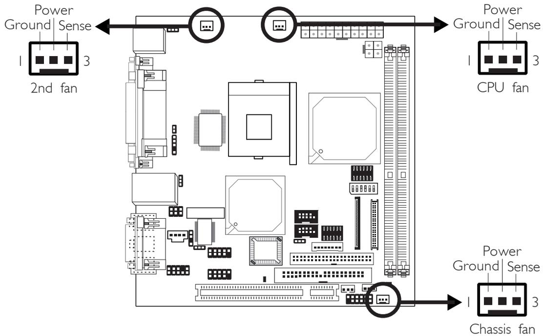
Connect the CPU fan's cable connector to the CPU fan connector (J2) on the system board. The chassis fan (J1) and 2nd fan (J3) connectors are used to connect an additional cooling fan. The cooling fans will provide adequate airflow throughout the chassis to prevent overheating the CPU and system board components.
