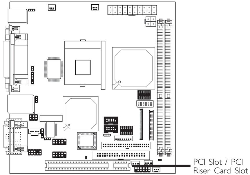
You can install a PCI expansion card or a customized riser card designed for 1, 2 or 3 PCI slots expansion (for low profile PCI card only).
