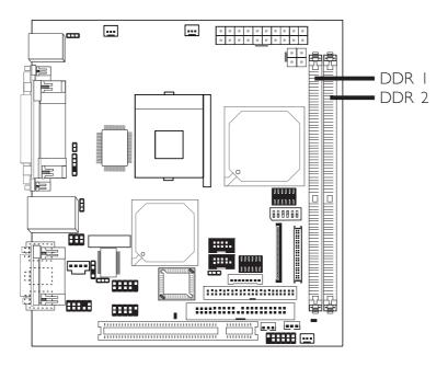
The system board supports DDR SDRAM DIMM. Double Data Rate SDRAM (DDR SDRAM) is a type of SDRAM that doubles the data rate through reading and writing at both the rising and falling edge of each clock. This effectively doubles the speed of operation therefore doubling the speed of data transfer.
