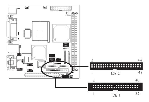
The system board is equipped with a 40-pin (IDE I) and a 44-pin (IDE 2) IDE connectors. To prevent improper IDE cable installation, the IDE I connector has a keying mechanism. The connector on the IDE cable can be inserted into IDE I only if pin I of the cable connector is aligned with pin I of IDE I.
