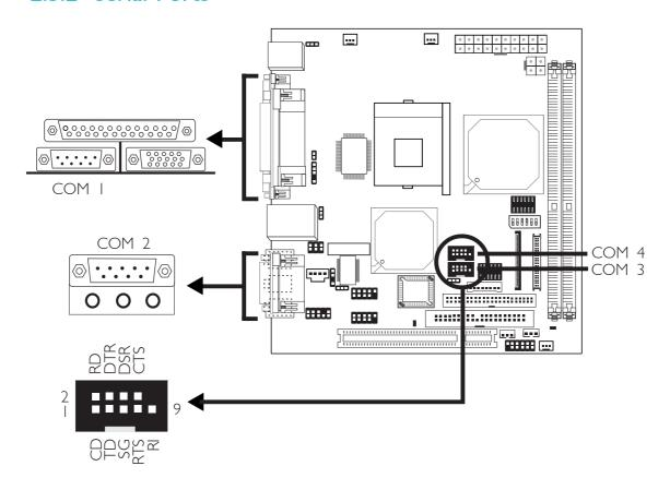
The system board is equipped with two onboard serial ports at locations CN13 (COM I) and CN14 (COM 2). It is also equipped with two 9-pin connectors at locations J14 (COM 3) and J15 (COM 4). These serial ports are RS-232 and/or RS-485 asynchronous communication ports with 16C550A-compatible UARTs that can be used with modems, serial printers, remote display terminals, and other serial devices.
