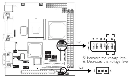
1-2 On: Increases the voltage level 2-3 On: Decreases the voltage level
