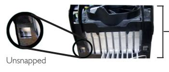
Fan / heat sink and retention mechanism assembly
