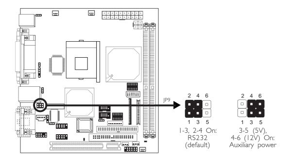
COM 2 is an RS-232 port. If the serial device connected to this port requires 5V/12V power from the system board, set JP9 pins 3-5 and 4-6 to On. Otherwise, leave this jumper's setting at 1-3, 2-4 On.
