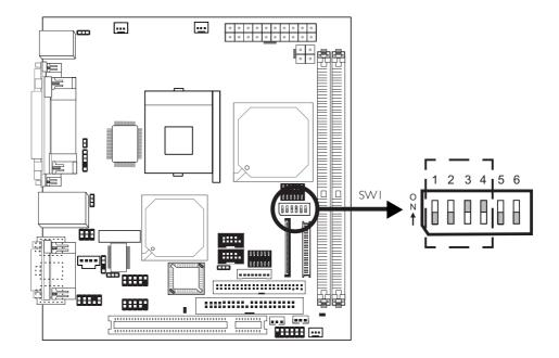
Set SWI pins I to 4 according to the type of LCD panel connected to the system. Please contact technical support for more information about the panel type settings.
