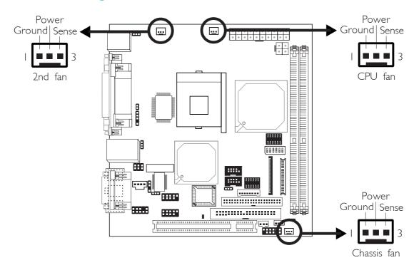
Connect the CPU fan's cable connector to the CPU fan connector (J2) on the system board. The chassis fan (J1) and 2nd fan (J3) connectors are used to connect an additional cooling fan. The cooling fans will provide adequate airflow throughout the chassis to prevent overheating the CPU and system board components.
