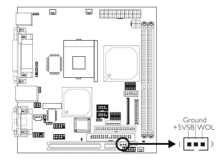
Your LAN card package should include a cable. Connect one end of the cable to the wakeup header on the card and the other end to location J12 on the system board. The network will detect Magic Packet and assert a wakeup signal to power-up the system. Refer to the add-in card's manual for details. Note: Your LAN card must support the remote wake up function.
