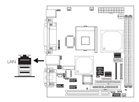
The system board is equipped with an onboard RJ45 LAN port. This port allows the system board to connect to a local area network by means of a network hub.
