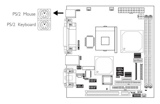
The system board is equipped with an onboard PS/2 mouse (Green) and PS/2 keyboard (Purple) ports - both at location CN5 of the system board. The PS/2 mouse port uses IRQ12. If a mouse is not connected to this port, the system will reserve IRQ12 for other expansion cards.
