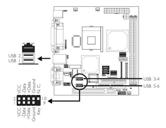
The system board supports 6 USB 2.0/1.1 ports. USB allows data exchange between your computer and a wide range of simultaneously accessible external Plug and Play peripherals.
