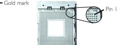
4. Insert the CPU into the socket until it is seated in place. The CPU will fit in only one orientation and can easily be inserted without exerting any force.
