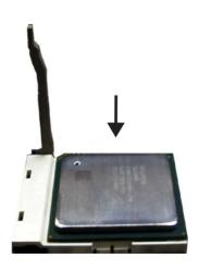
5. Once the CPU is in place, push down the lever to lock the socket. The lever should click on the side tab to indicate that the CPU is completely secured in the socket.
