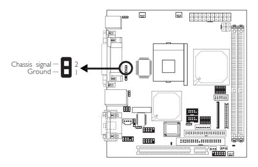
The system board supports the chassis intrusion detection function. Connect the chassis intrusion sensor cable from the chassis to J8. Whenever a chassis component has been removed, the sensor sends signal to J8 alerting you of a chassis intrusion event. To disable this function, place a jumper cap over J8.
