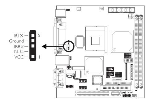
Connect your IrDA cable to connector |4 on the system board.
