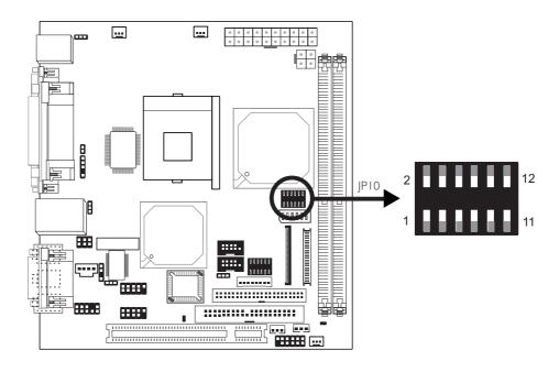
JP10 is used to select the power supplied to the LCD panel as well as configure the inverter.
