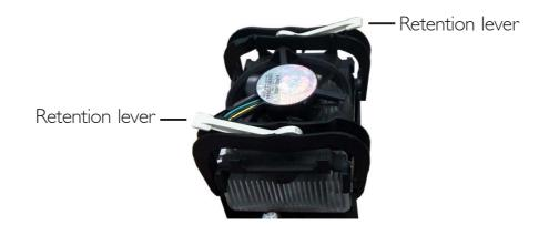
4. Move the retention levers to their opposite directions then push them down. This will secure the fan / heat sink and retention mechanism assembly to the retention module base.
