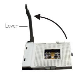
3. Position the CPU above the socket then align the gold mark on the corner of the CPU (designated as pin I) with pin I of the socket.
