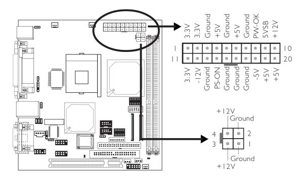
Use a power supply that complies with the ATX12V Power Supply Design Guide Version I.I. An ATX12V power supply has a standard 20-pin ATX main power connector and a 4-pin +12V power connector that must be inserted onto CN10 and CN1 connectors respectively.
