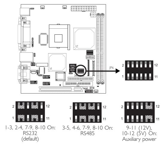
JP6 is used to set COM 4 to RS-232 or RS-485. If the serial device connected to this port requires 5V/12V power from the system board, set JP6 pins 9-11 and 10-12 to On. This setting automatically sets COM 4 at RS-232.
