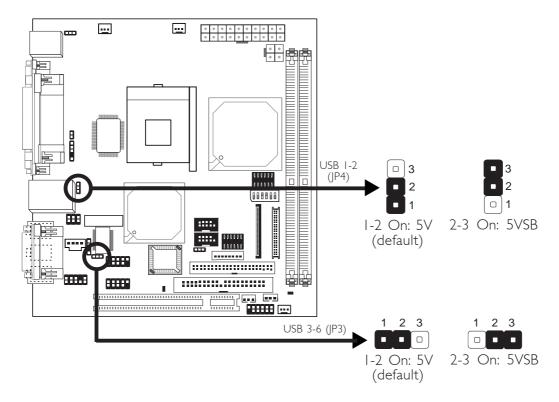
JP4 (for USB I-2) and JP3 (for USB 3-6) are used to select the power of the USB ports. Selecting 5VSB will allow you to use the USB keyboard or USB mouse to wake up the system.
