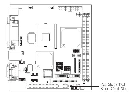
You can install a PCI expansion card or a customized riser card designed for I, 2 or 3 PCI slots expansion (for low profile PCI card only).
