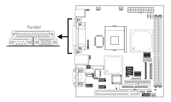
The system board has a standard parallel port (Burgundy) at location CN3 for interfacing your PC to a parallel printer. It supports SPP, ECP and EPP.
