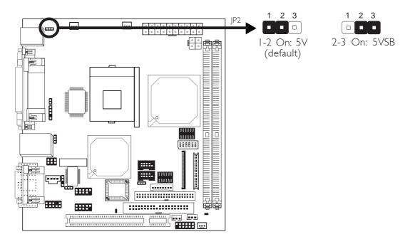
JP2 is used to select the power of the PS/2 keyboard/mouse port. Selecting 5VSB will allow you to use the PS/2 keyboard or PS/2 mouse to wake up the system.
