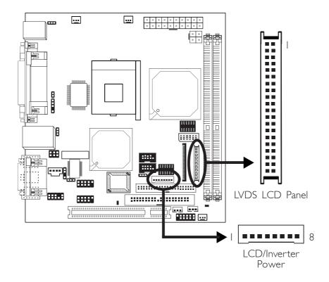
The system board allows you to connect a LCD Display Panel by means of the LVDS LCD panel connector (CN12) and the LCD/Inverter power connector (CN11). These connectors transmit video signals and power from the system board to the LCD Display Panel. Refer to the next page for the pin functions of these connectors.
