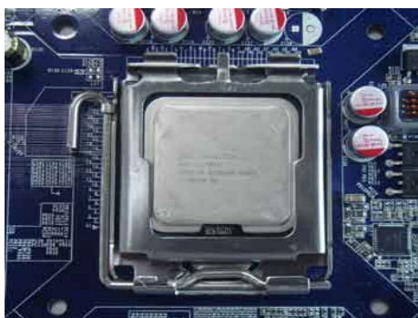
5. When CPU is properly seated, replace the metal cover and push the CPU socket lever back to its locked position.
