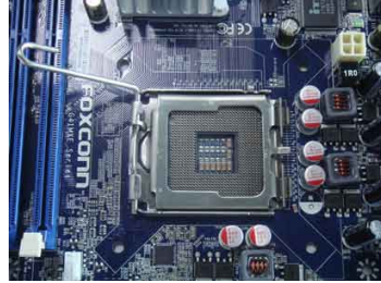
2. Release the CPU socket lever.
