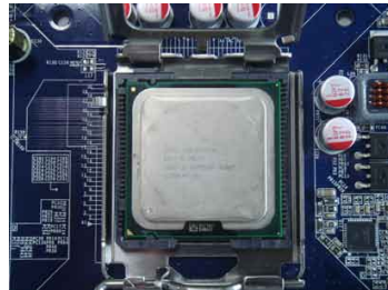
4. Check pin one marking (triangle) with the pin one corner of the CPU socket, align the CPU notches with the socket alignment keys and gently put the CPU onto the socket.
