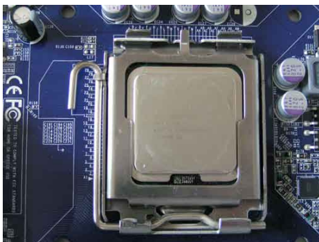
5. When CPU is properly seated, replace the metal cover and push the CPU socket lever back to its locked position.
