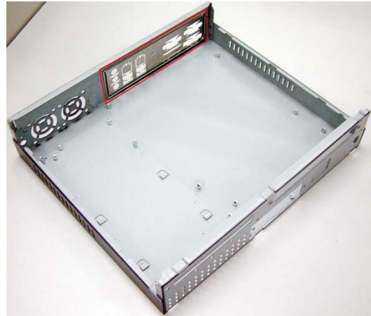
2. Set the F04-137-F I/O shield to the side of the chassis.
