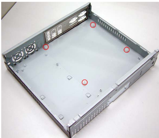
3. Put the space-support holders on the four pillars.
