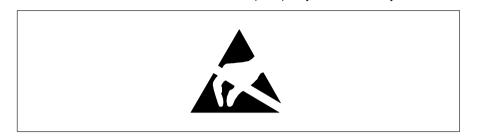
Modules with electrostatic sensitive devices (ESD) may be identified by labels.
