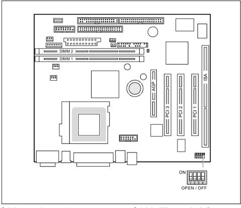
Switch 1 = must be set to *off* Switch 2 = System BIOS recovery (RCV) Switch 3 = Write protection for floppy disks Switch 4 = reserved
