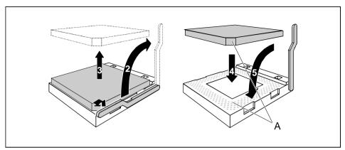
The heat sink is mounted on the processor with a clip.
