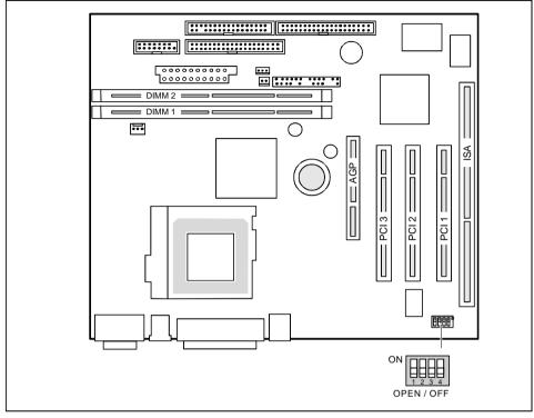
Switch 1 = must be set to *off* Switch 2 = System BIOS recovery (RCV) Switch 3 = Write protection for floppy disks
