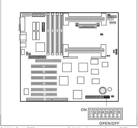
Switch 1 = System BIOS recovery Switch 2 = must be set to *off*  Switch 3 = write protection for system BIOS Switch 4 = write protection for floppy disk drive Switch 5, 6, 7, 8 = clock frequency
