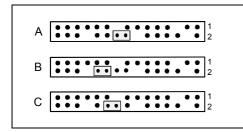
Pin pair A inserted = Skipping system and BIOS Setup password
