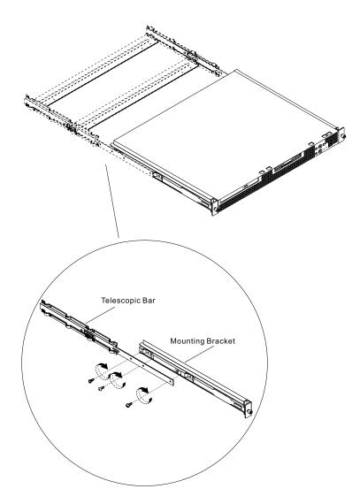
2 The left and right mounting bracket share a common part. Thus, a mounting bracket could be used as either a left or right mounting bracket depending on how you turn it around.
