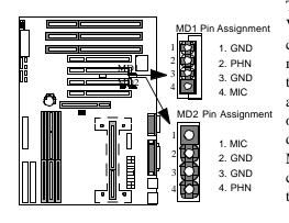
This 1x4 header is used for Voice Modem's internal connector. This allows modem's voice can be direct to the onboard sound chip and amplified by speaker. The pin out and connect type are different between MD1 and MD2. MD1 is a JST type connector and MD2 is a MPC2 type connector.
