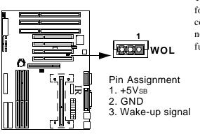
This 3-pin header is used for remote wake up of the computer through a network card with WOL function.
