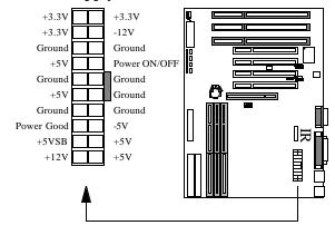
The ATX power supply has a single lead connector with a clip on one side of the plastic housing. There is only one way to plug the lead into the ATX power connector. Press the lead connector down until the clip snaps into place and secures the lead onto the connector
