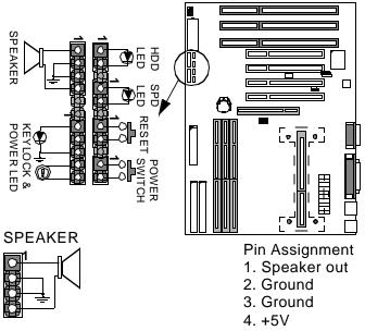
This 4-pin connector connects to the case-mounted speaker.
