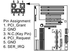
This 2x3 ways, straight-3 header is used for Creative Lab PCI sound card (Ex. AWE64D PCI Audio Wave Table Card). In order to migrate the legacy Sound Blaster compatible audio to the PCI bus, the following signals have to be delivered to the PCI audio card through a flat cable.
