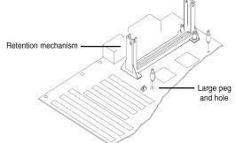
2. Slide a black plastic support onto each end of the fan or heatsink, making sure that the hole and clip are on the outside edge of the support. (If supports are reversed, the holes will not line up with the pegs on the motherboard.) Slide each support toward the center of the processor until the support is seated in the outside groove of the fan housing.
