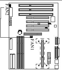
Pin Assignment 1. GND 2. +12V 3. SPEED / RPM
