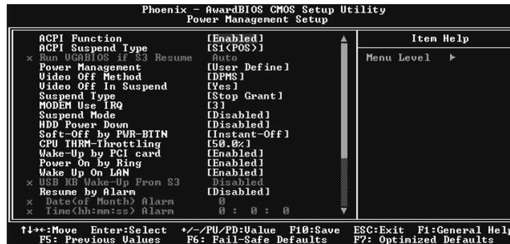
**ACPI Function :** When set to “Enabled”, turns on the ACPI Function . The default setting is “Disabled”.
