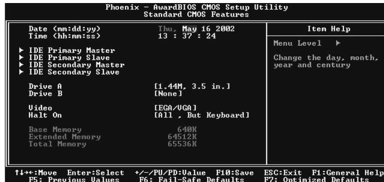
The Standard CMOS Setup utility is similar for all three chipsets and is used to configure the following features:
