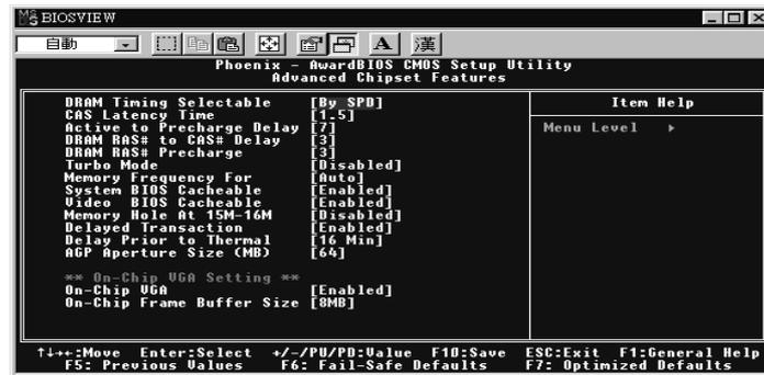
This option displays a table of items that define critical timing parameters of the mainboard. You should leave the items on this page at their default values unless you are very familiar with the technical specification of your system hardware. If you change the values incorrectly, you may introduce fatal errors or recurring instability into your system.
