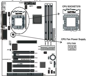
2. Push the CPU socket lever slightly to the side and then raise it as far as it can go.
