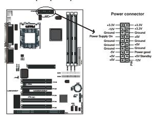
**Warning:** Incorrect installation of the power supply could result in serious damage to the mainboard and connected peripherals. Make sure the power supply is unplugged from the AC outlet before connecting the leads from the power supply.
