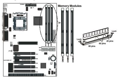
You must use 3.3V unbuffered DIMMs in the mainboard. To determine the DIMM type, check the notches on the DIMMs.
