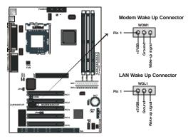
Note: You must enable the Wake On LAN/Wake On Modem features in the BIOS setup if you use this feature. Refer to the Power Management section in Chapter 4 for details.
