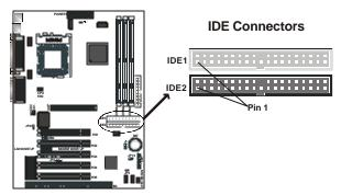
Consult the documentation that came with your IDE drive for details on jumper locations and settings. You must orient the cable connector so that the pin 1 (color) edge of the cable corresponds to pin 1 of the I/O port connector.
