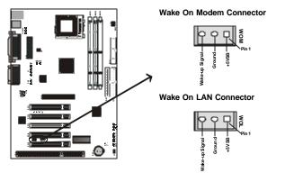
Note: You must enable the Wake On LAN/Wake On Modem features in the BIOS setup if you use this feature. Refer to the Power Management section in Chapter 4 for details.
