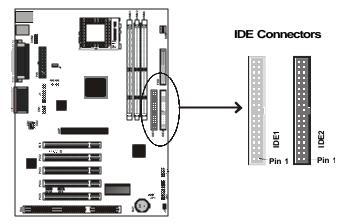
Consult the documentation that came with your IDE drive for details on jumper locations and settings. You must orient the cable connector so that the pin 1 (color) edge of the cable corresponds to pin 1 of the I/O port connector.
