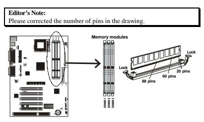
You must use 3.3V unbuffered DIMMs in the mainboard. To determine the DIMM type, check the notches on the DIMMs.
