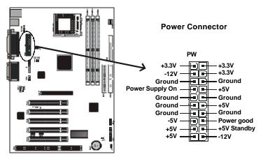
**Warning:** Incorrect installation of the power supply could result in serious damage to the mainboard and connected peripherals. Make sure the power supply is unplugged from the AC outlet before connecting the leads from the power supply.
