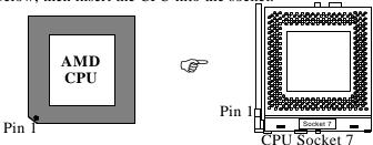
3. Press the lever down to snap it into place at the side of socket. You will feel some resistance as the pressure starts to secure the CPU in the socket.
