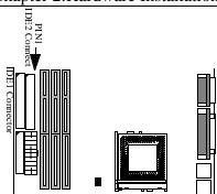
Consult the documentation that comes with your IDE drive for details on jumper locations and settings. You must orient the cable connector so that the pin 1(color) edge of the cable is at the pin 1 of the I/O port connector.
