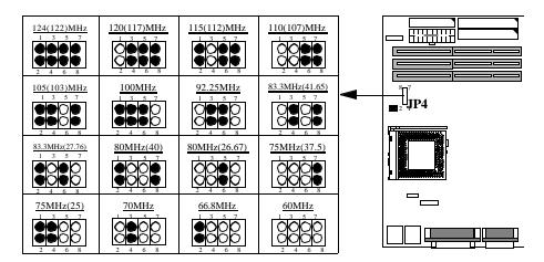
Warning: The VIA MVP4 chipset supports maximum 100MHz external CPU bus clock, if you want your system running at over-frequency 112MHz, you should have faster SDRAM, PCI add on card and good heat dissipation CPU fan. Otherwise, that may cause your system to become unstable. We recommend you to use the standard CPU frequency for normal operation.
