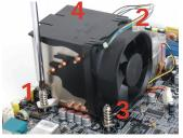
**3** The cooler dock is especially designed to allow an elastic connection with the CPU. Please slide the coole rover the four position pins of the dock, andthen use a screwdriver to tighten the cooler to the dock, as shown in the illustrations.
