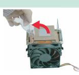
1 Take off the transparent plastic cover from the bottom of the cooler. Please do not touch the thermal grease in the center of the bottom.
