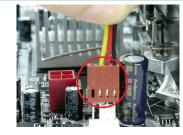
**5** Connect the Fan cable onto the CPU FAN connector onboard.
