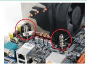
**4** Note that the four screws should be completely through the cooler, and tightly connected with the dock.
