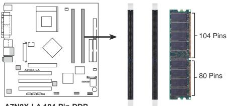
A7N8X-LA 184-Pin DDR DIMM Sockets
