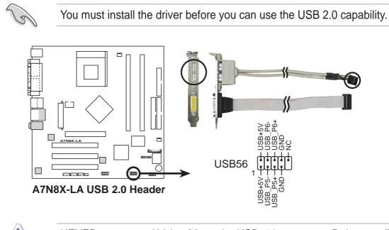
NEVER connect a **1394 cable** to the USB\_56 connector. Doing so will damage the motherboard!
