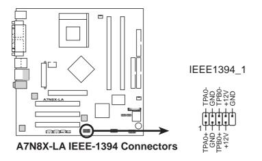
NEVER connect a **USB cable** to any of the IEEE 1394 connectors. Doing so will damage the motherboard!
