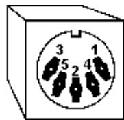
5-Pin Keyboard Connector
