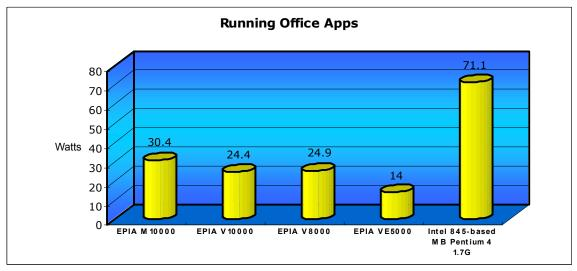
The comparison above uses CC Winstone 2001 to compare power consumption while carrying out standard office tasks like word processing, manipulating spreadsheets and database work. In this comparison, the fanless VIA EPIA VE5000 mainboard uses around 20% of the power used by the reference platform.
