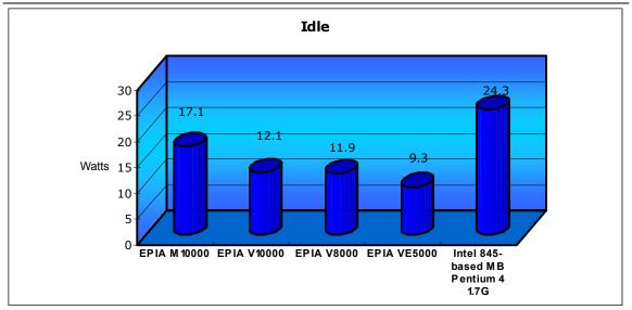
In this comparison, the power consumed while standing idle is compared and the VIA EPIA V-Series mainboards draw around 35% of the power that the Intel reference platform draws.
