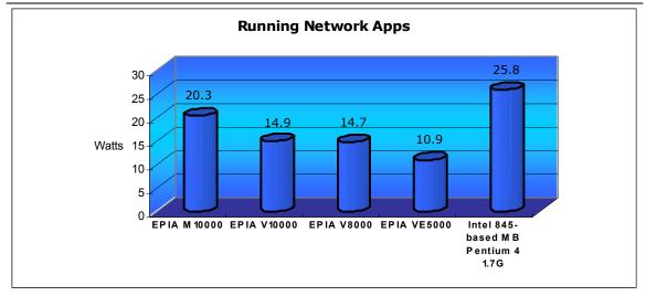
The power consumption comparison for network applications was run while transferring large data files over a standard 10 Base T network. Here again the power consumption of the Intel reference platform is considerably more than that of the VIA EPIA V-Series with the EPIA VE5000 drawing less than 40% of the power of the reference platform.
