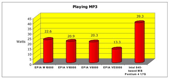
Power consumption of EPIA V's flagship V10000 is only half of that of the reference platform. The fanless VIA EPIA VE5000 uses a meager 33% of the power that the reference platform. This is significant as power sensitive systems like in-car MP3 systems are gaining in popularity.
