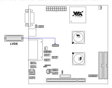
The LVDS-05 module is equipped with the VIA VT1631 transmitter. It provides a way to connect to LCD panel displays. It supports 24-bit MSB LCD panels. The native resolution is  $1024 \times 768$ .
