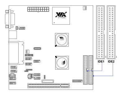
If two drives are connected to a single cable, the jumper on the second drive must be set to slave mode. Refer to the drive documentation supplied by the vendor for the jumper settings.
