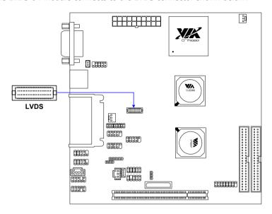
The LVDS-04 module is equipped with the VIA VT1631 transmitter. It provides a way to connect to LCD panel displays. It supports 18-bit LSB LCD panels. The native resolution is  $1024 \times 768$ .
