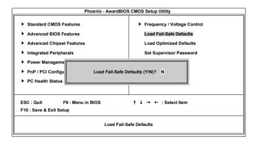
This option is for restoring all the default fail-safe BIOS settings. These values are set by the mainboard manufacturer to provide a stable system with basic performance.
