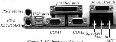
Figure 3: I/O back panel layout
