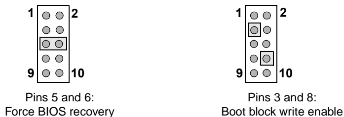
Figure 2-2. BIOS configuration jumper block settings
