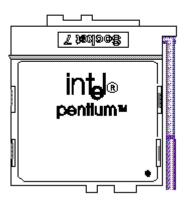
2. Intel Pentium 90MHz (P54C/P54CT/P54CTB) CPU (60MHz Host Clock) installed on board
