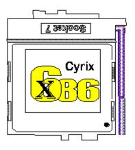
13. Cyrix 6X86 120MHz CPU (60MHz Host Clock) installed on board
