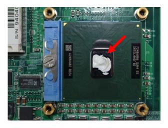
Figure 3-9: How to Install CPU (3)
