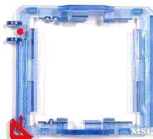
3. Align the 3 points (the Pin 1 indicator and the two alignment keys) of both the CPU and the CPU Clip, and use your 4 fingers to push the CPU Clip down to clip them (the CPU clip is up and the CPU is down) together.
