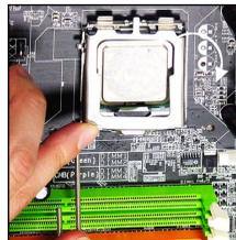
13. Press down the load lever lightly onto the load plate, and then secure the lever with the hook under retention tab.
