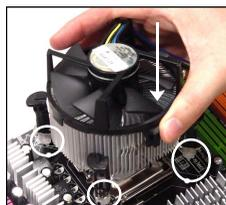
15. Press the four hooks down to fasten the cooler. Then rotate the locking switch (refer to the correct direction marked on it) to lock the hooks.
