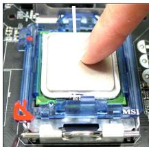
12. Visually inspect if the CPU is seated well into the socket, then remove the CPU Clip with 2 fingers. Then cover the load plate onto the package.
