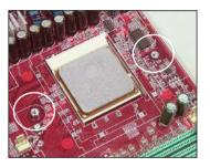
4. Align the retention mechanism and the backplate.
