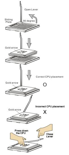
5. Press the CPU down firmly into the socket and close the lever. As the CPU is likely to move while the lever is being closed, always close the lever with your fingers pressing tightly on top of the CPU to make sure the CPU is properly and completely embedded into the socket.
