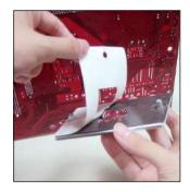
2. Turn over the mainboard, and install the backplate to the proper position.
