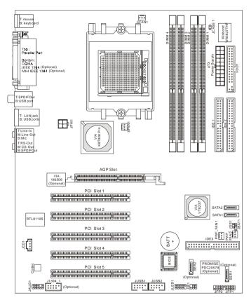
K8T Neo2 (MS-6702E) v1.X ATX Mainboard
