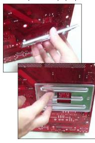
5. Position the cooling set onto the retention mechanism.
