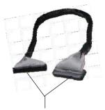
Connect one end to the floppy disk drive connector (FDD1) and the other end to the standard floppy disk.
