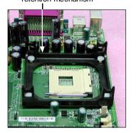
Position the heatsink onto the retention mechanism.
