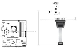
P7H55-M Serial port (COM1) connector
