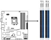
P7H55-M 240-pin DDR3 DIMM sockets
