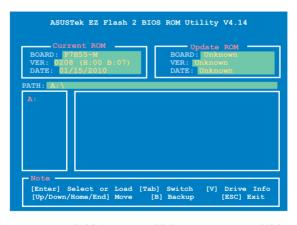
When the correct BIOS file is found, EZ Flash 2 performs the BIOS update process and automatically reboots the system when done.
