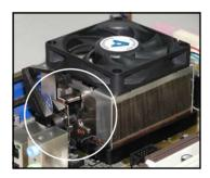
Push down the retention bracket lock on the retention mechanism to secure the heatsink and fan to the module base.
