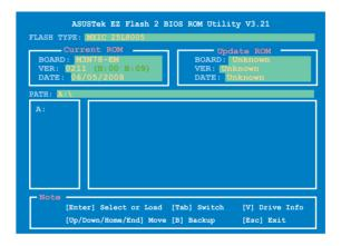
(2) Enter BIOS setup program. Go to the **Tools** menu to select **EZ Flash 2** and press <Enter> to enable it.
