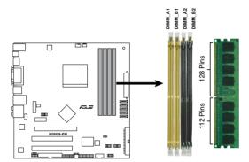
M3N78-EM 240-pin DDR2 DIMM Sockets
