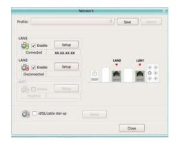
If you use a network cable connected to a home router (which is then connected to your DSL/cable modem), enable both LAN1 and LAN2. Express Gate will automatically use whichever port (LAN1 or LAN2) is connected.
