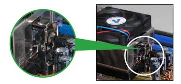
Align the other end of the retention bracket (near the retention bracket lock) to the retention module base. A clicking sound denotes that the retention bracket is in place.
