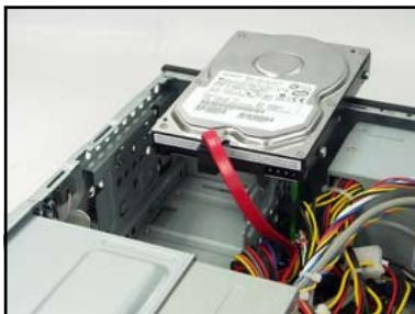
4. Connect the 15-pin SATA power plug from the power supply unit to the power connector at the back of the drive.
