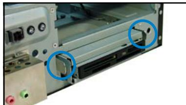
3. Press the card reader lock inwards(A), then slightly pull the card reader assembly outward (B) until the USB cable and plug is exposed.
