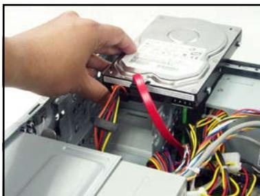
5. Place the HDD on the tray. Make sure that the HDD screws are aligned with the screw holes and rails.
