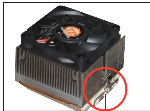
Socket tabs matched to the holes on the heatsink bracket
