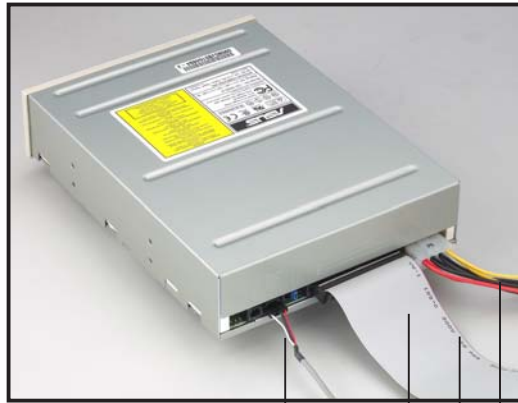
Optical drive audio cable IDE ribbon cable Red stripe to Pin 1 Power cable
