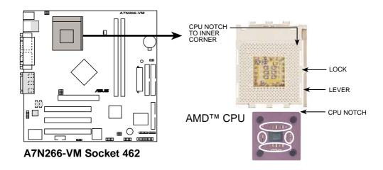
Each AMD CPU has a "marked" corner. This corner is usually indicated with a notch, and/or a golden square or triangle. Refer to this indicator while orienting the CPU. See the next page for installation details.
