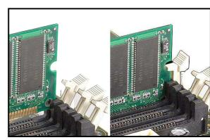
Unlocked Retaining Clip Locked Retaining Clip
