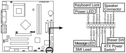
A7N266-VM System Panel Connectors\* Requires an ATX power supply.
