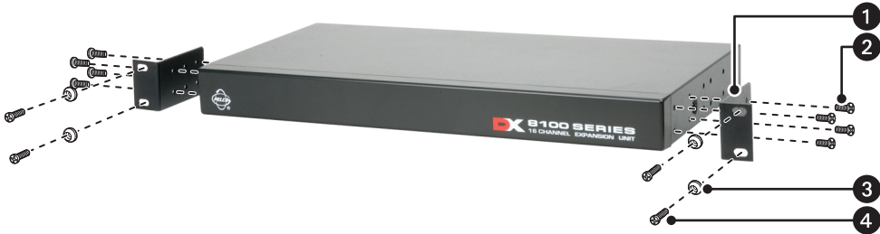
Figure 14. Assembling Expansion Unit Rack Mount Kit
