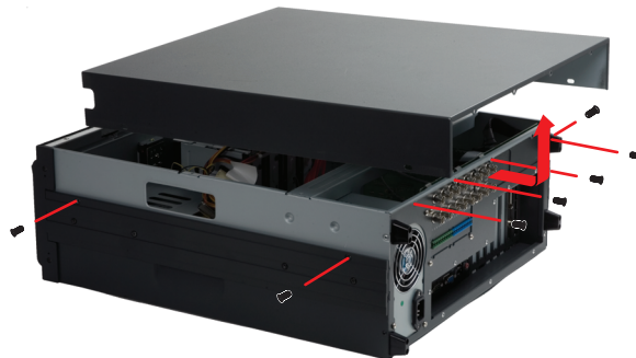
Figure 6. Removing Chassis Cover
