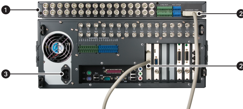
Figure 15. Interfacing the Expansion Unit and DX8100
