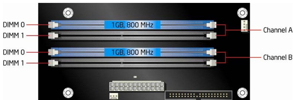
Figure 17. Dual Channel Memory Configuration with Two DIMMs
