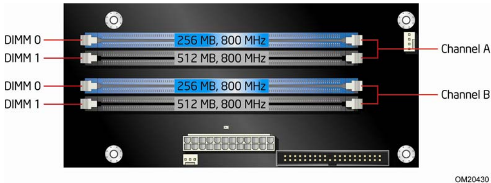
Figure 18. Dual Channel Memory Configuration with Four DIMMs
