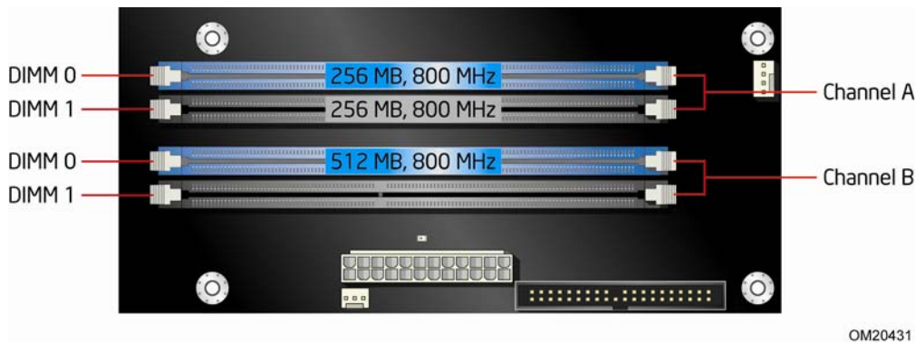
Figure 19. Dual Channel Memory Configuration with Three DIMMs
