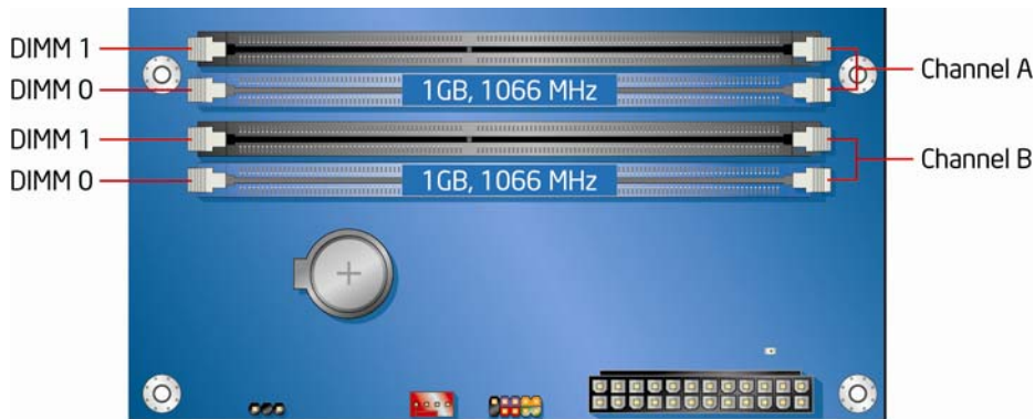
Figure 14. Example Dual Channel Memory Configuration with Two DIMMs
