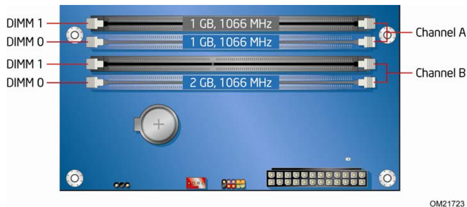
Figure 16. Example Dual Channel Memory Configuration with Three DIMMs
