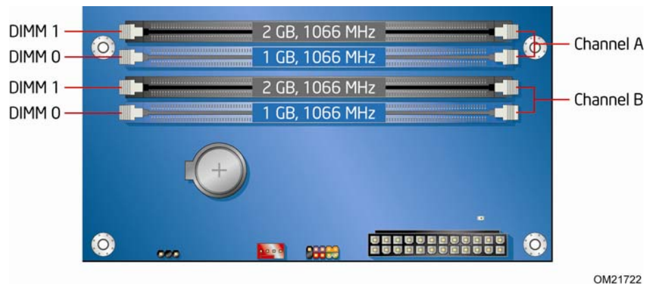
Figure 15. Example Dual Channel Memory Configuration with Four DIMMs
