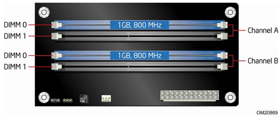
Figure 14. Dual Channel Memory Configuration with Two DIMMs
