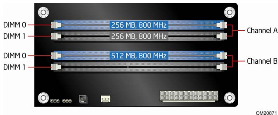
Figure 16. Dual Channel Memory Configuration with Three DIMMs
