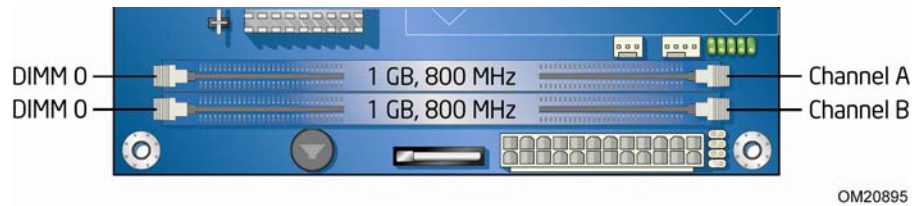
Figure 13. Dual Channel Memory Configuration Example
