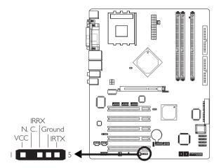
Connect your IrDA cable to connector J22 on the system board.
