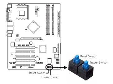
The presence of the reset switch and power switch on the system board are user-friendly especially to DIY users. They provide convenience in powering on and/or resetting the system while fine tuning the system board before it is installed into the system chassis.
