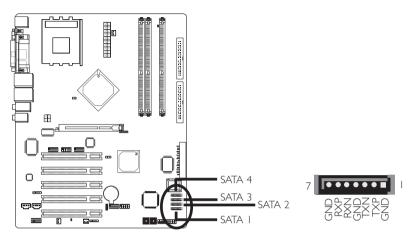
The system board is equipped with 4 SATA connectors at locations J18 (SATA 1), J17 (SATA 2), J16 (SATA 3) and J15 (SATA 4) for connecting SATA devices. Connect one end of the SATA cable to a SATA connector and the other end to your SATA device.
