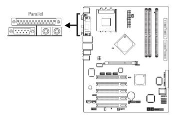
The system board has a standard parallel port (Burgundy) at location CN9 for interfacing your PC to a parallel printer. It supports SPP, ECP and EPP.
