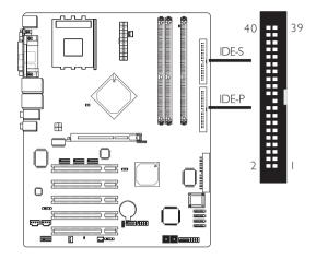
The system board is equipped with two shrouded PCI IDE headers that will interface four Enhanced IDE (Integrated Drive Electronics) disk drives. To prevent improper IDE cable installation, each shrouded PCI IDE header has a keying mechanism. The 40pin connector on the IDE cable can be placed into the header only if pin I of the connector is aligned with pin I of the header.
