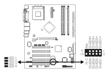
The 4 diagnostic LEDs on the system board are used to indicate the current condition of the system.
