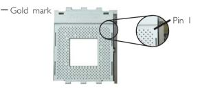
6. Insert the CPU into the socket until it is seated in place. The CPU will fit in only one orientation and can easily be inserted without exerting any force.
