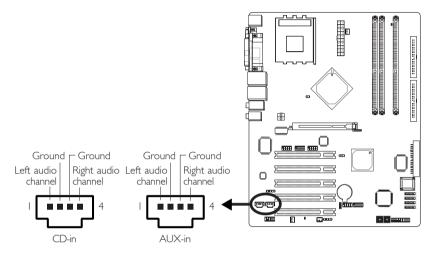
The CD-in (J1) and AUX-in (J3) connectors are used to receive audio from a CD-ROM drive, TV tuner or MPEG card.
