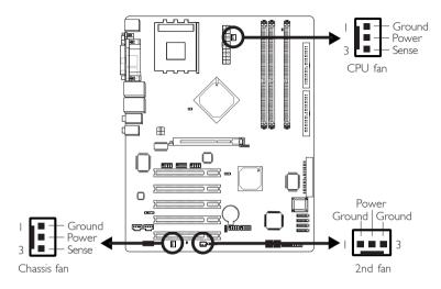
Connect the CPU fan's cable connector to the CPU fan connector (J11) on the system board. The chassis fan (J6) and 2nd fan (J10) connectors are used to connect additional cooling fans. The cooling fans will provide adequate airflow throughout the chassis to prevent overheating the CPU and system board components.
