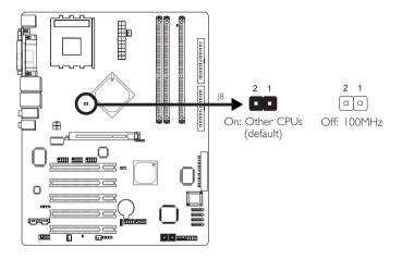
This jumper is used to select the front side bus of the CPU installed on the system board.
