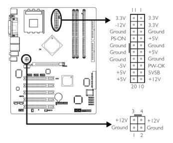
We recommend that you use a power supply that complies with the ATX12V Power Supply Design Guide Version 1.1. An ATX12V power supply has a standard 20-pin ATX main power connector and a 4-pin +12V power connector that must be inserted onto CN11 and CN10 connectors respectively.
