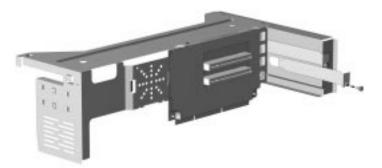
Removing the Screw and Expansion Slot Cover
