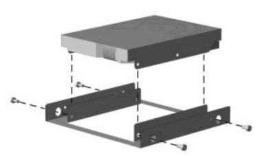
Attaching a 3.5-Inch Drive to the 5.25-Inch Bracket
