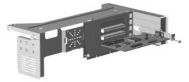
Removing a Graphics Controller from a PCI Expansion Slot
