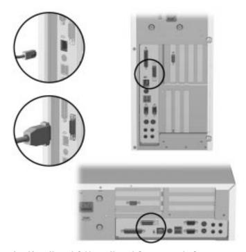
Attaching a Network Cable to a Network Connector on the Computer
