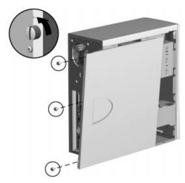
Loosening the Thumbscrews and Removing the Side Panel
