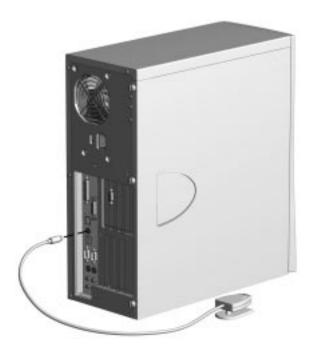
Connecting an External Infrared Transceiver
