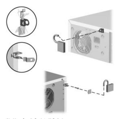
Attaching a Security Bracket with Padlock
