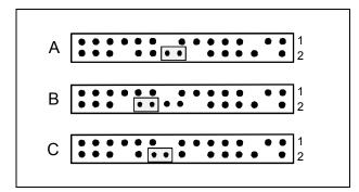
Pin pair A inserted = Skipping system and BIOS Setup password
