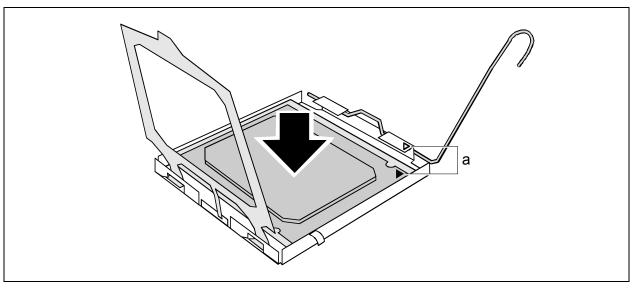
Insert the new processor in the socket so that the marking of the processor is aligned with the marking on the socket (a).
