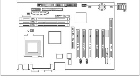
Switch 1 = must be set to *off* Switch 2 = System BIOS recovery Switch 3 = Write-protection for floppy disk Switch 4 = must be set to *off*
