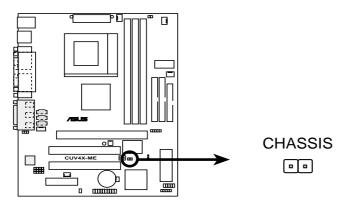
**CUV4X-ME Chassis Open Alarm Lead**
