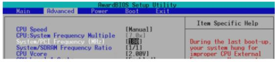
Cause for Hangup: Improper System/SDRAM Frequency Ratio
