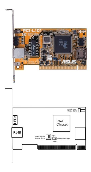
If you are using the ASUS PCI-L101 on an ASUS motherboard, leave the jumper on its defaut setting of "ASUS." If you are using another brand of motherboard, set the jumper to "Other." Connect the Wake on LAN (WOL) output signal to the motherboard's WOL\_CON in order to utilize the wake on LAN feature of the motherboard. Connect the LAN activity output signal (LAN\_LED) to the system cabinet's front panel LAN\_LED in order to display the LAN data activity.
