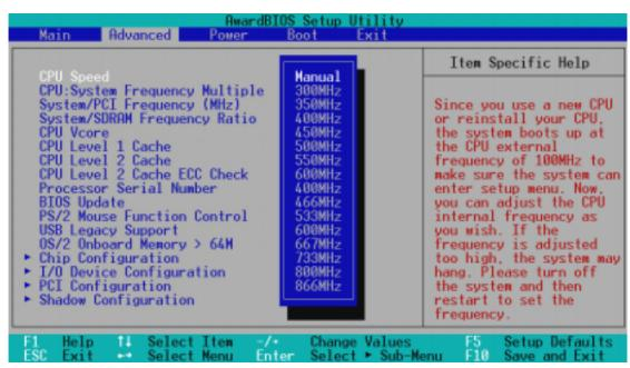
For processors with unlocked frequency multiplier
