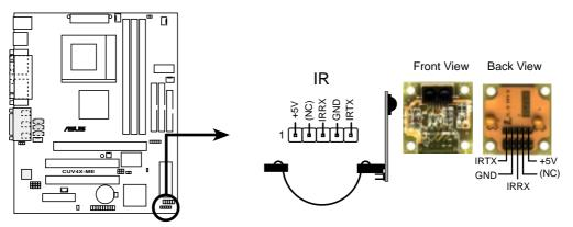
**CUV4X-ME Infrared Module Connector**
