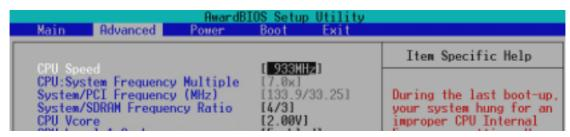
Cause for Hangup: Improper CPU Speed
