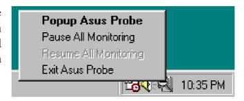
When the ASUS PC Probe senses a problem with your PC, portions of the ASUS PC Probe icon changes to red, the PC speaker beeps, and the ASUS PC Probe monitor appears.
