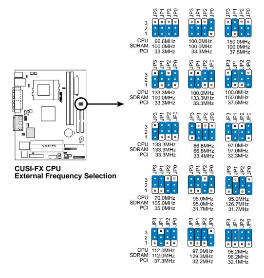
**Manual CPU Settings** (**NOTE:** JumperFree mode must be disabled.) *Set the jumpers according to the internal speed of your processor as follows:*
