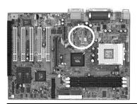
This board includes a VGA ports riser which is to be connected to this header.
