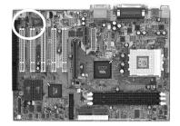
This connector is for Surround and Center+Bass speaker output ext. Plug in the optional AC3 Surround/Center+Bass jack extension into this connector. The black colored jack is for surround speaker output and the orange colored jack is for center+bass speaker output.
