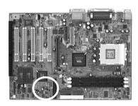
This board supports the chassis instruction monitoring feature of the management extension hardware by means of a mechanical or photo sensor switch attached to the motherboard through this 1x3-pin chassis security header. The mechanical switch is set to open for normal computer operation.
