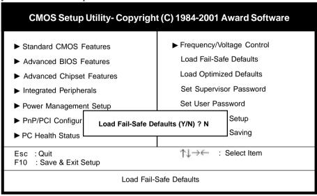
Figure 3-10 Load Fail-Safe Defaults Screen
