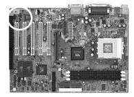
The S/PDIF-out connector supports the digital audio. This connector must be connected to the cable from an external device (i.e.2-channel decoded AC-3 from DVD decoders).
