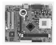
Use the auxiliary audio cable enclosed with your CD-ROM disk drive to connect the CD-ROM to your mainboard. This will enable your CD-ROM's audio function.
