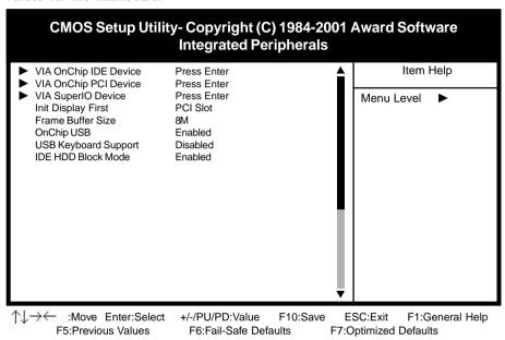
Figure 3-5 Integrated Peripherals Screen
