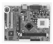
This connector is use for front panel audio jack ext. and is to be connector into a special custom designed system case.
