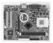
This connector is to be connected to an optional TV-out/DFP adapter card.
